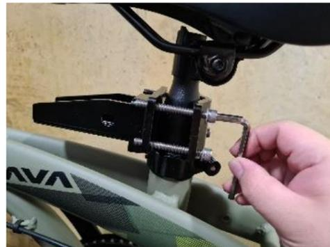
**5** Assemble the seat by raising the paw deck and securing the center stand with the blue labelled M4 screws and washers.
