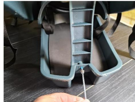
**6** Flip your Buddyrider seat upside and align the support arm's holes with the Buddyrider seat's holes. Position the Buddyrider seat on the support arm as far forward as possible without causing any interference with the steering post or handlebars of the bicycle.
