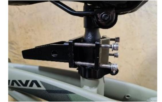
**4** Install the receiver as high up the seat pole as possible. Tighten the 4 M6 screws with washers using the hexagon key.
