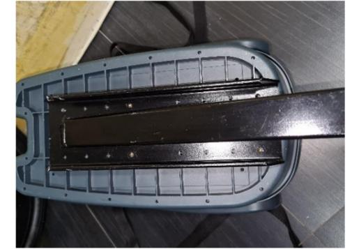
**7** Tighten the remaining 4 red labelled screws using the hexagon key.
